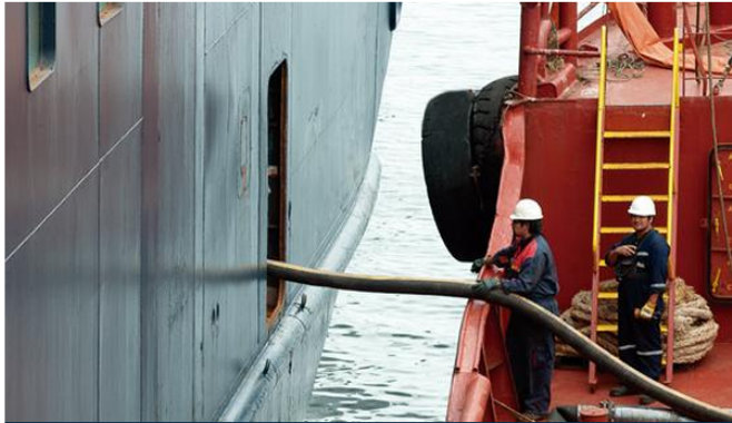
BUNKER TRANSFER OPERATIONS
